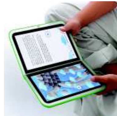
› The second generation of OLPC machines are expected to feature dual touch screens.
