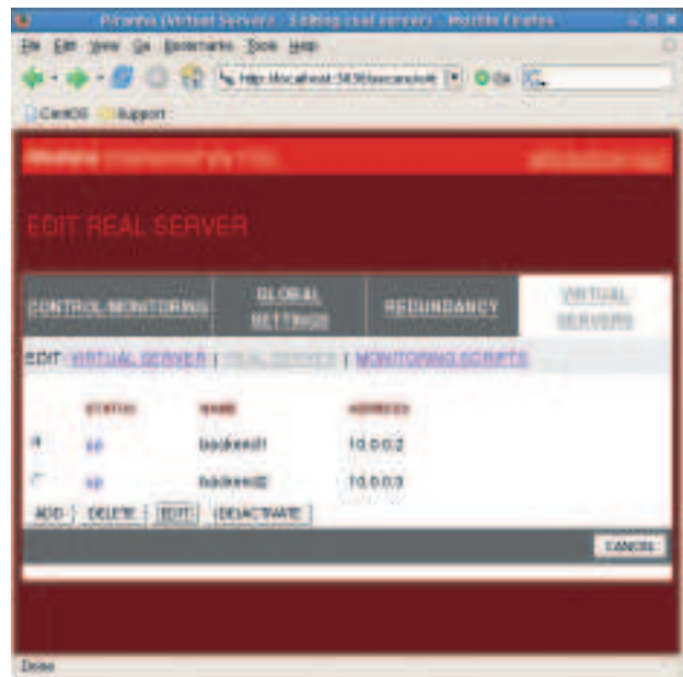
Figure 3: Specifying the real (backend) servers.
